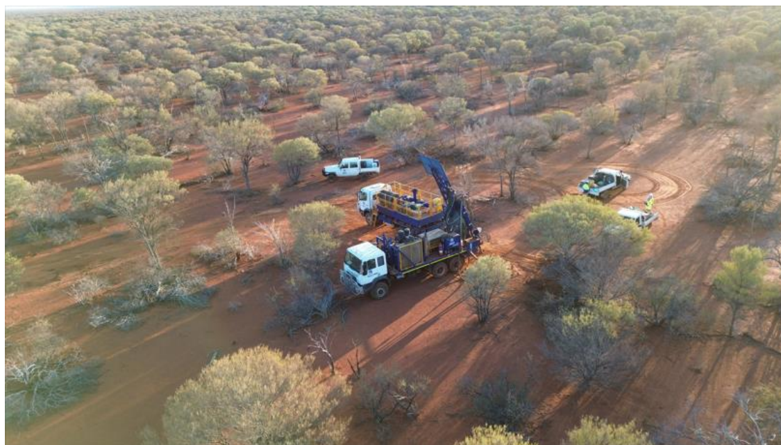
Figure 1: Aircore drilling in soil-covered terrain at Bunjarra.
