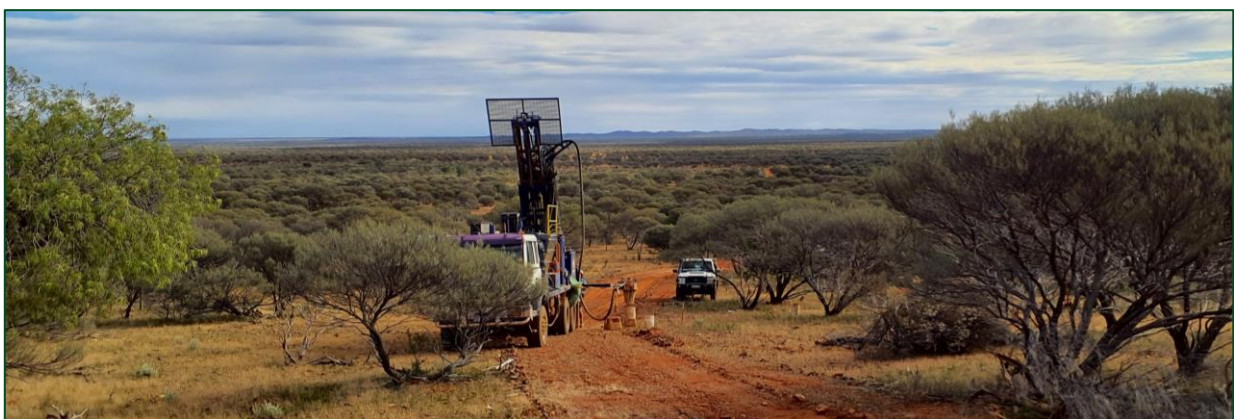
Figure 4: Reconnaissance aircore drilling in typical shallow colluvial terrain at Box Soak.
