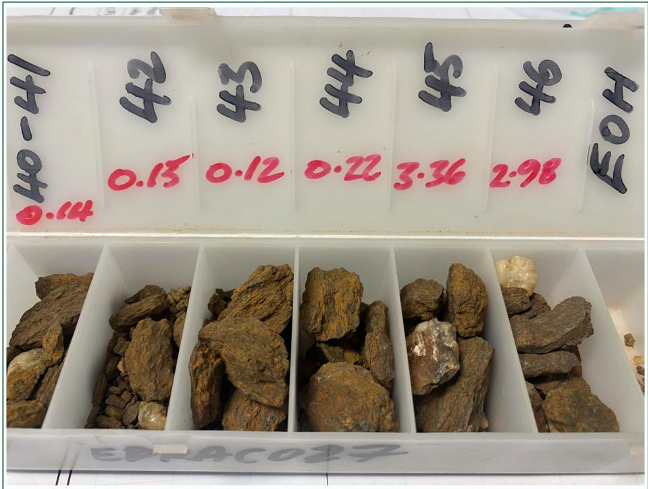
Figure 2: Photo of EDRAC027 chip tray with 1m samples 40m to 46m EOH and gold assay (g/t Au) results labelled in iron altered schist and quartz veining.
