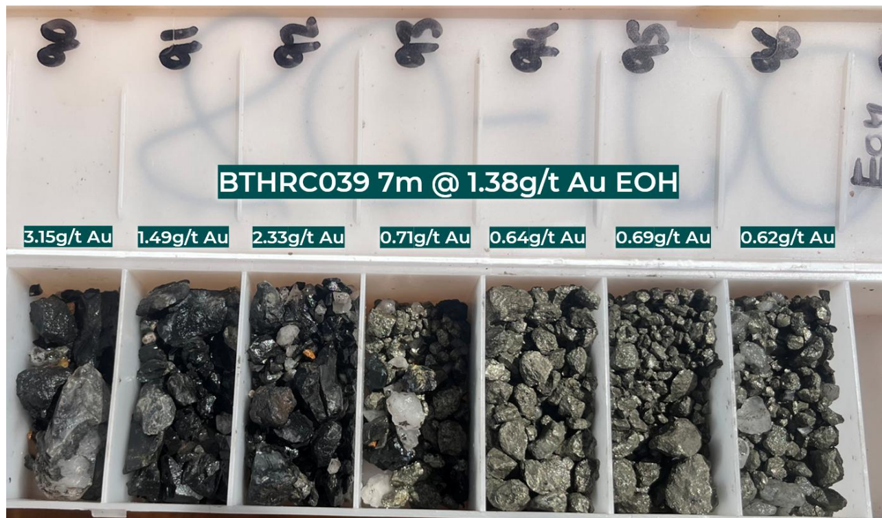
Figure 4: Photo of BTHRC039 chip tray with 1m intervals and gold grades from 89m to 96m EOH. Geology changes from chert and quartz veining, into quartz veining and massive pyrite toward end of hole.
