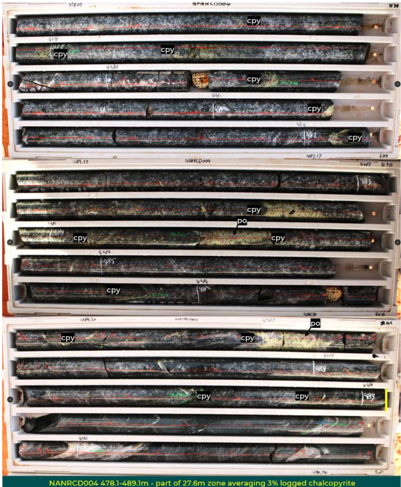
Photo 3. Core tray photos of gabbro from 478.1m to 489.1m (11.0m), with chalcopyrite (cpy) and pyrrhotite (po) sulphide zones labelled. These trays are part of a 27.6m zone averaging 3% logged visual* chalcopyrite (Table 1).
