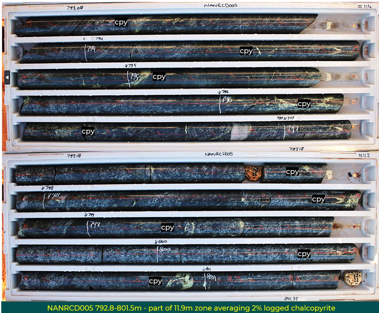
Photo 5. Core tray photo of altered gabbro from 792.8m to 801.5m (8.7m), with chalcopyrite (cpy) sulphide zones labelled. This tray is part of a 11.9m zone averaging 2% logged visual chalcopyrite* (Table 1).
