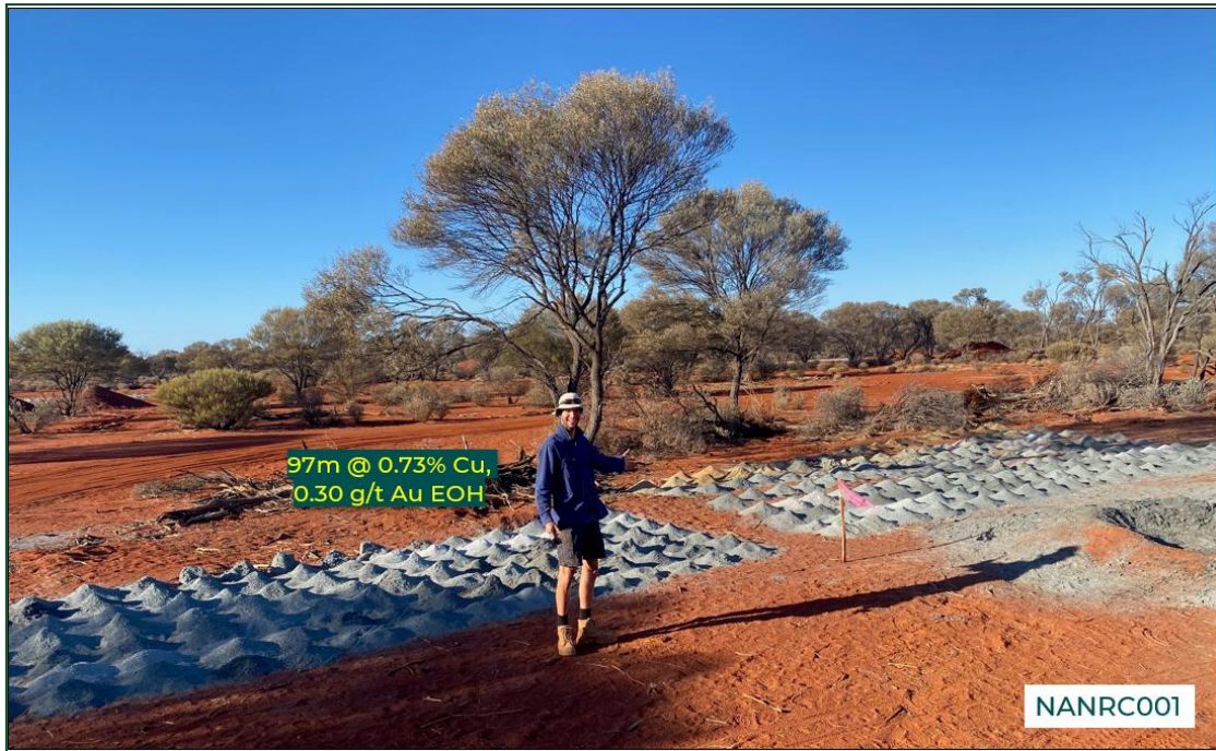
Photo 2. Typical RC drill samples (NANRC001) 1 at Nanadie. Note the limited oxidation profile below shallow sandy soils.
