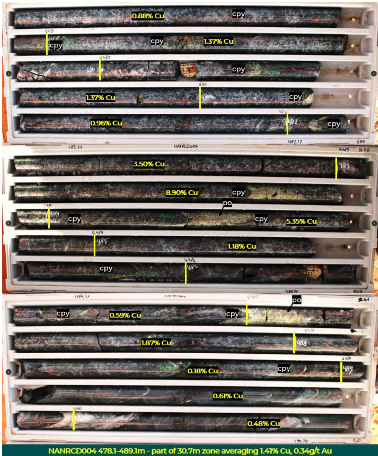
Photo 1. Core tray photos of altered gabbro from 478.1m to 489.1m (11.0m), with chalcopyrite (cpy) and pyrrhotite (po) sulphide zones labelled alongside copper assays. These trays are part of a 27.6m zone that was logged as averaging 3% logged visual chalcopyrite 2 that has subsequently returned an intercept of 30.7m @ 1.41% Cu and 0.34g/t Au from 461.5m
