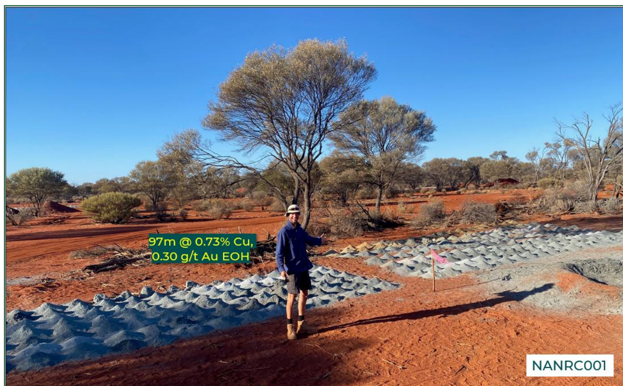
Photo 1. Typical RC drill samples (NANRC001) at Nanadie 1 . Note the limited oxidation profile below shallow sandy soils.
