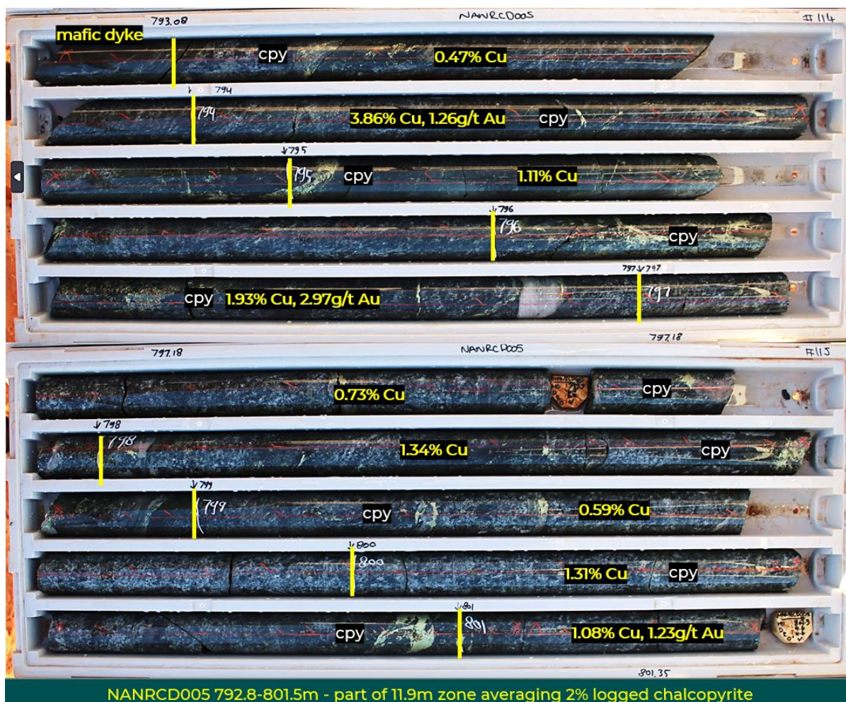
Photo 1. Core tray photos of altered gabbro from 792.8m to 801.5m (8.7m), with chalcopyrite (cpy) sulphide zones labelled alongside copper assays and gold assays where greater than 1g/t Au. These trays are part of a 43.3m zone that has subsequently returned an intercept of 0.91% Cu and 0.35g/t Au from 761.7m.
