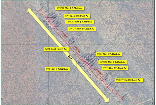
Figure 8. Statesman Well plan view showing all drillhole traces, significant results and untested segments of the mineralised surface.
