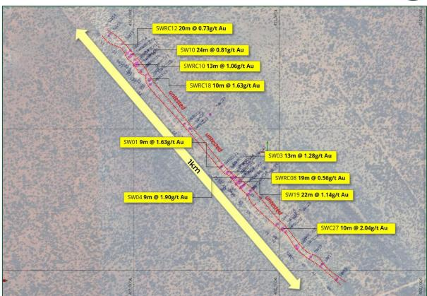
Figure 10. Statesman Well plan view showing all drillhole traces, significant results and untested segments of the mineralised surface<sup>18</sup>.
