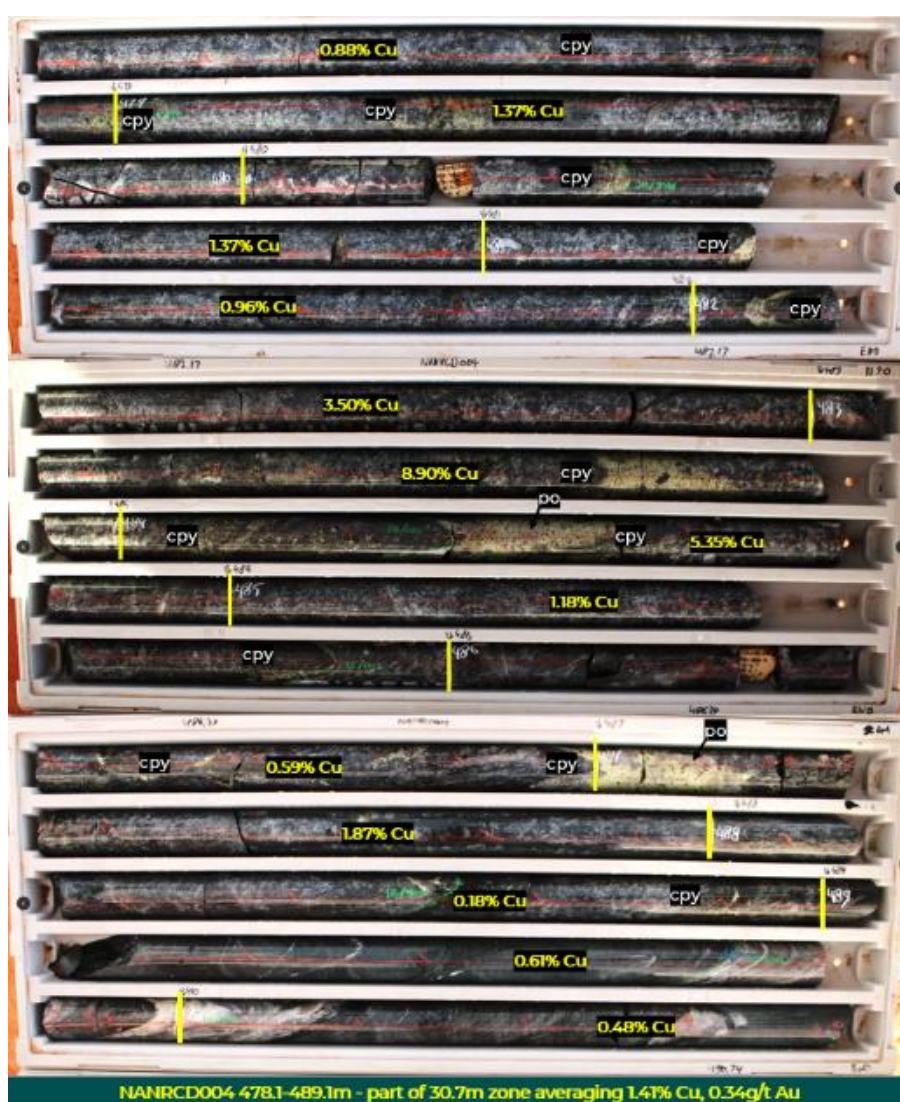
Photo 1. Core tray photos of altered gabbro in NANRCD004 from 478.1m to 489.1m (11.0m), with chalcopyrite (cpy) and pyrrhotite (po) sulphide zones labelled alongside copper assays 1 . These trays are part of a 27.6m zone that was logged as averaging 3% logged visual chalcopyrite 3 that has subsequently returned an intercept of 30.7m @ 1.41% Cu and 0.34g/t Au from 461.5m
